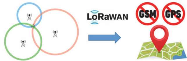
Fig. 1. LoRaWAN geolocation based on time of flight analysis of the packages sent from a low power IoT device. No GPS or GSM units were used.
