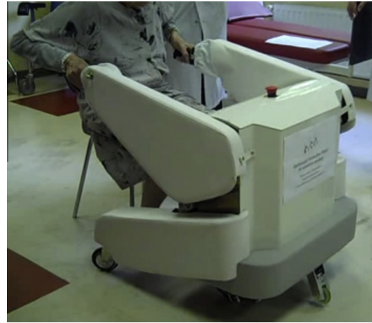
Fig. 1. MIRAS robot prototype during clinical investigation.
