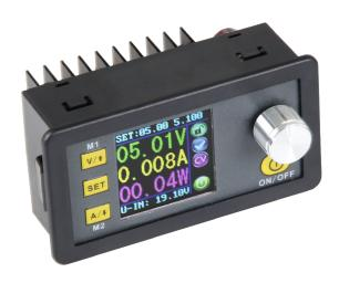
This programmable constant voltage and constant current control module combines analog integration and digital control functions in one device.
