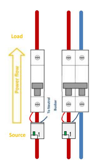
Smart Energy Sensor / Monitor with Wireless-communication for 1P+N System
