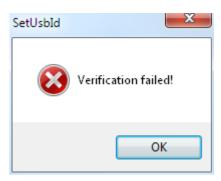
Action: check that the EEPROM write protection is enabled. Refer to the DLP® Discovery™ documentation about this.
